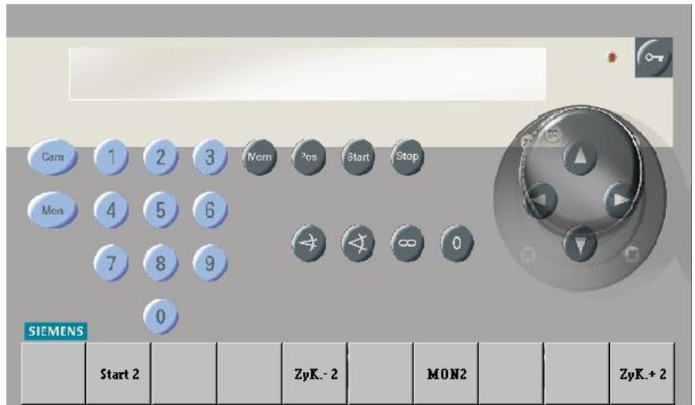
Fig. 19 Keyboard 2 (key layout CKAx; identical to keyboards 3 and 4; each device controls a single monitor)
